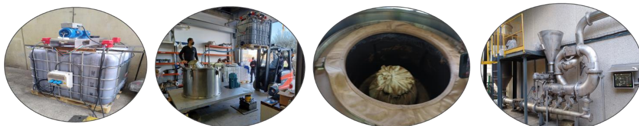
Figure 16. The steps established for the drying of the hydrolysed grape stem. From left to right: hydrolysis tank; centrifugation (outside and inside view); flash drying of the solid sample.
