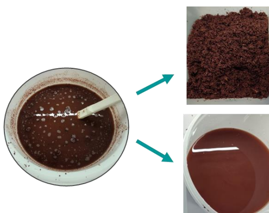
Figure 5. Washing process and the solid and liquid fractions obtained.
