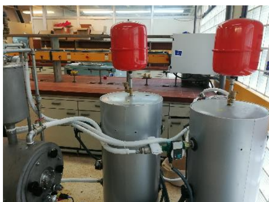
Figure 15. Main components of the heating system of the bioreactors
