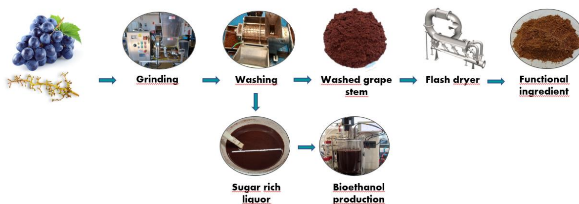
Figure 1. Proposed diagram for valorising grape stems from wineries.
